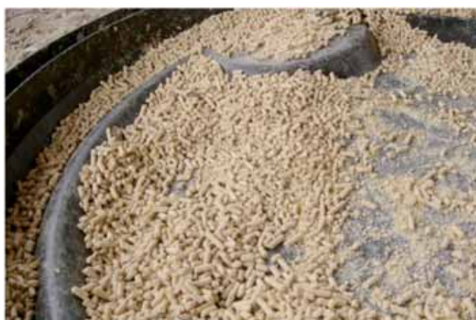
FIGURE 25 Locally pelleted feed in China [Note the high level of disintegrated pellets and dust]
